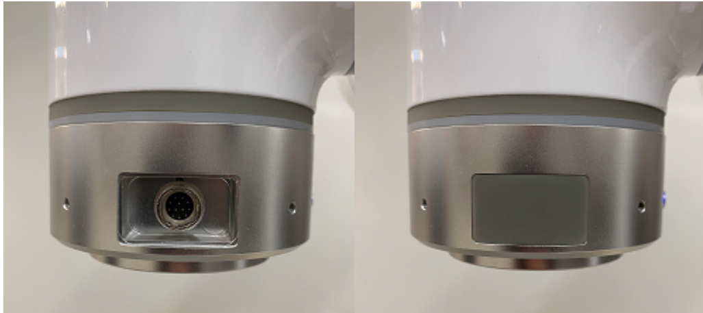
Figure 3-6 : Location of the Tool I/O plug
