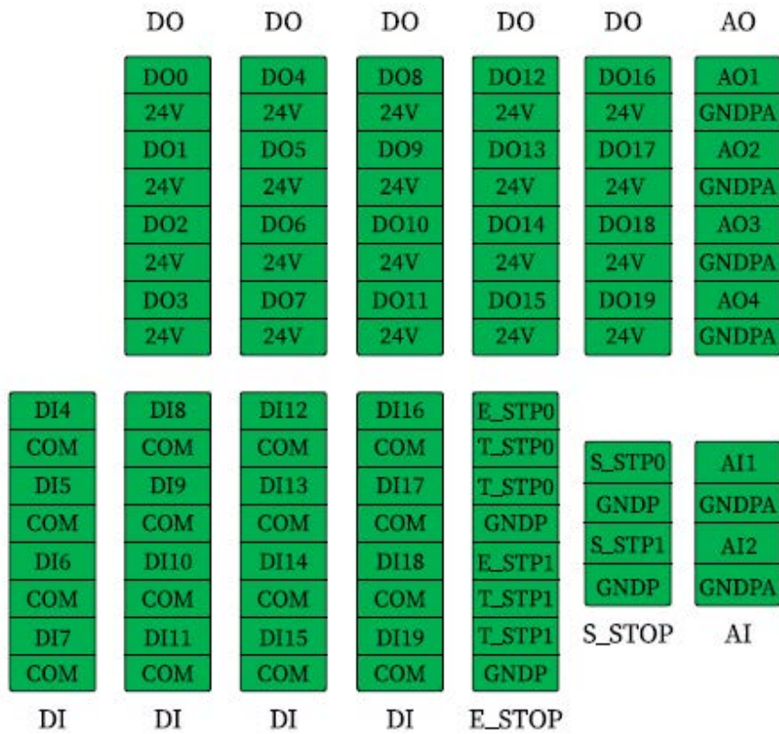
Figure 7-2 : The layout of the electrical interfaces inside the controller
