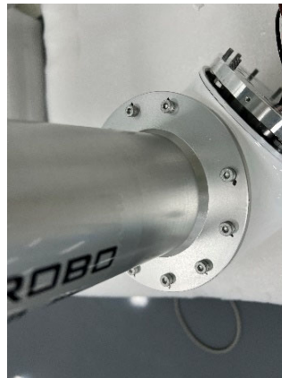
Figure 3-19 : Removing the upper arm supporting ring
