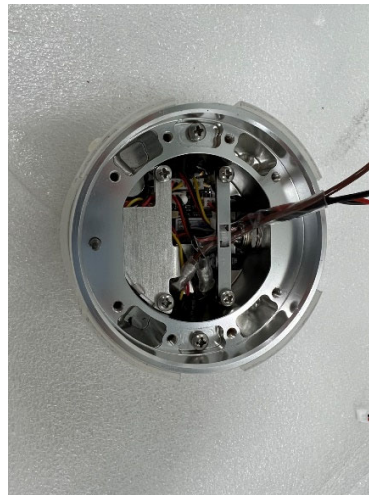
Figure 3-27 : Connecting wires between the wrist 3 joint and the tool flange
