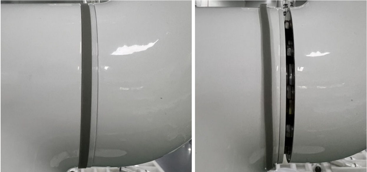
Figure 3-4 : Remove the rubber ring
