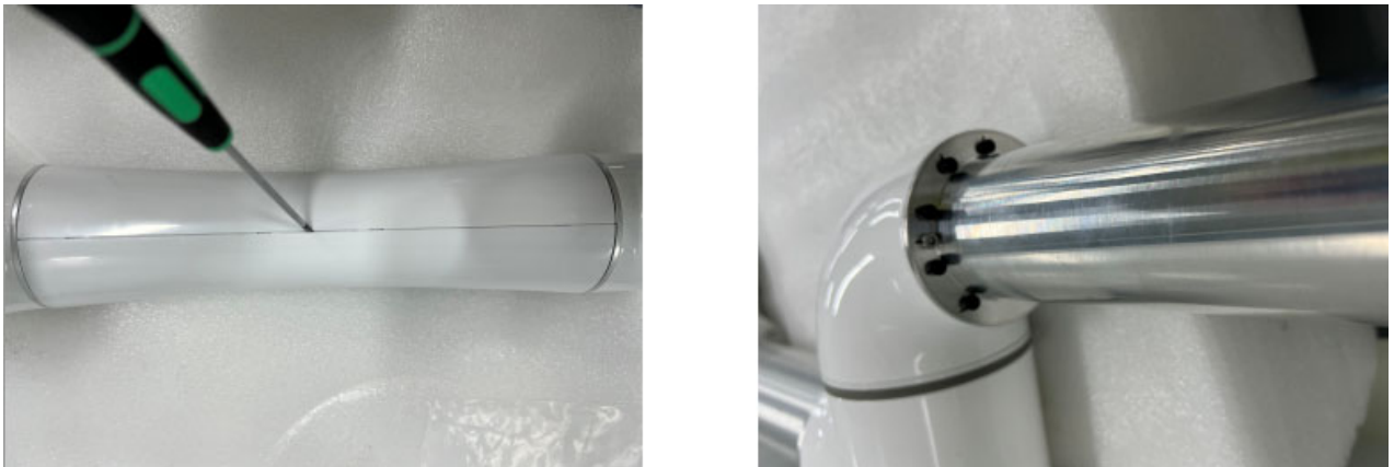
Figure 3-24 : Drawing wires connecting the wrist 2 joint
