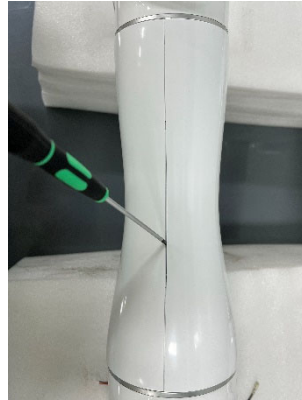
Figure 3-18 : Removing the rubber ring
