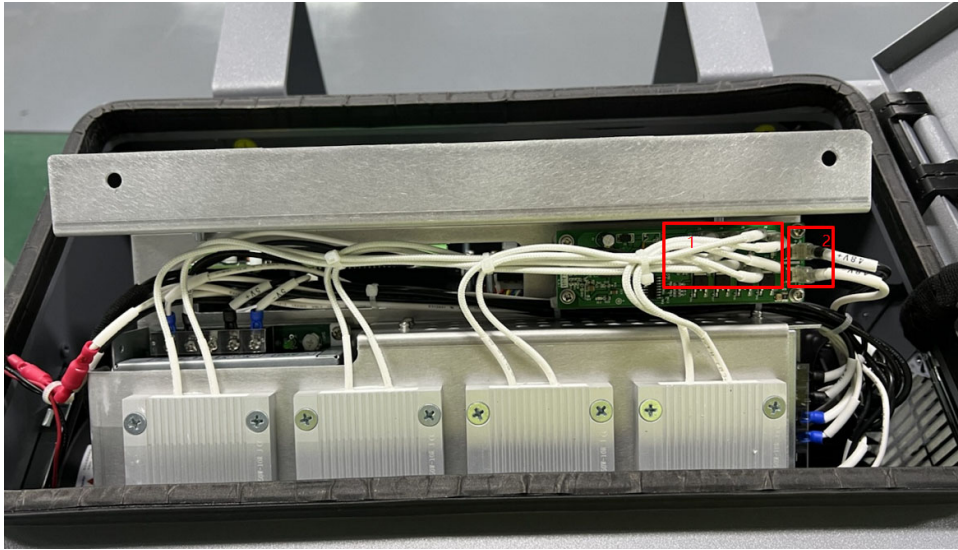
Figure 3-39 : Disconnect the wires
