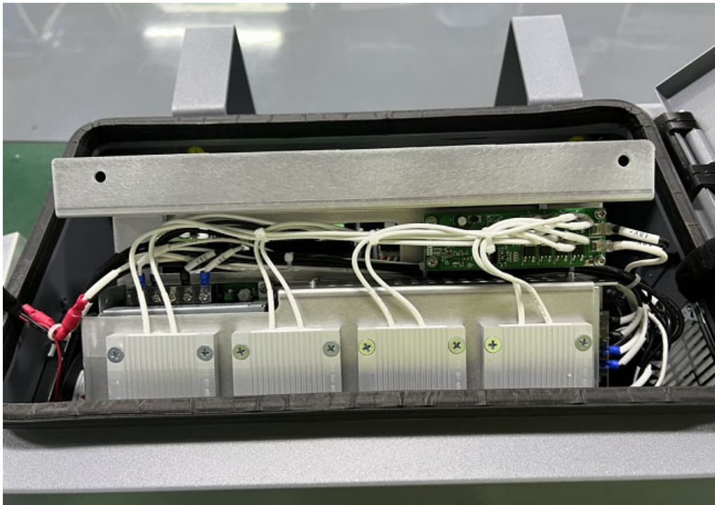
Figure 3-41 : Reconnect the cables
