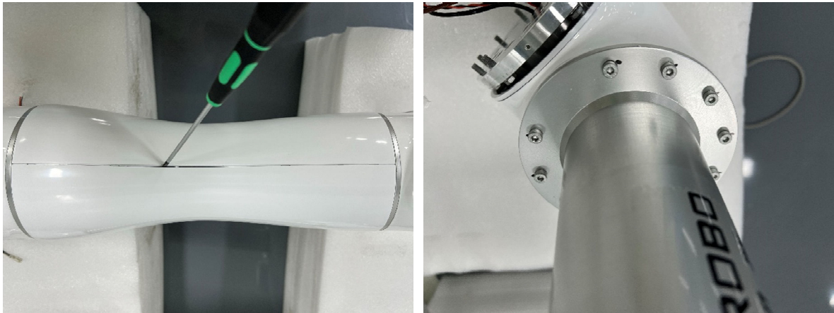
Figure 3-21 : Unscrew hex screws connecting the elbow joint and the upper arm link
